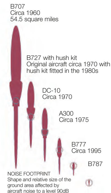
Figure 5.2: Shape and relative size of the ground area affected by aircraft noise (to a level of 90dB(A)) for different generations of Boeing aircraft
